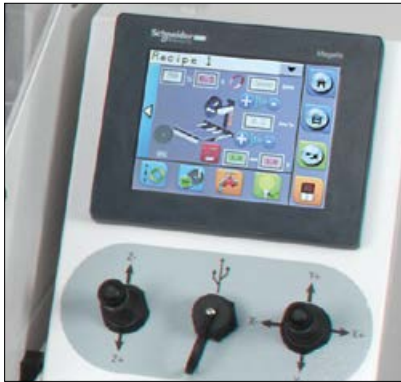
Quick positioning with joysticks. Touch screen with graphical interface.
